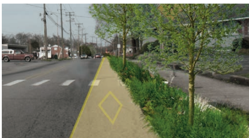
Figure 3.10: Some street retrofitted with linear bioretention, bike lane, and street trees (Source: SMART Center).
